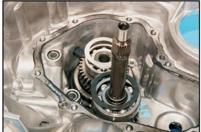
The front reduction drive & driven gears can now be removed.
