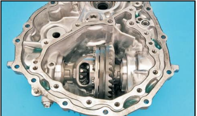
The converter case also houses the final drive carrier.
